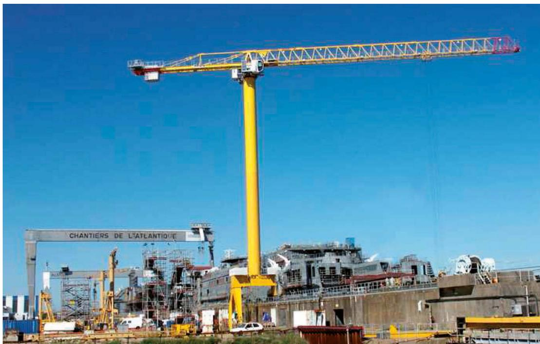
The previously Alstom Marine division - Chantiers de l'Atlantique company ordered a MDT crane with a special 20 t capacity to work under a giant overhead travelling crane. The use of the topless technology enables maximum possible height under hook.
